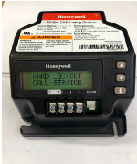
HARD LOCKOUT AFTER 2 RESETS (3 LOCKOUTS) AFTER THE 3RD SUCCESSIVE HARD LOCKOUT THE CONTROL WILL SET A RESTRICTED HARD LOCKOUT AND DISPLAY THE "CALL SERVICE" MESSAGE. THE BURNER SHOULD BE CHECKED BY QUALIFIED PERSONNEL TO DETERMINE WHY THE BURNER FAILS TO FIRE OR IS NOT FUNCTIONING PROPERLY.
