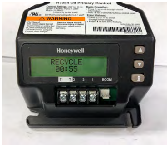
CONTROL IN 60 SEC. RECYCLE AFTER A FLAME LOSS OR SIMILAR INTERRUPTION DURING NORMAL FIRING & CALL FOR HEAT.
