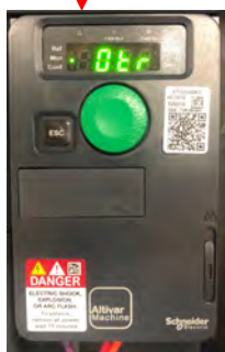
MOTOR TORQUE(ESTIMATED) 100% = NOMINAL MOTOR TORQUE
