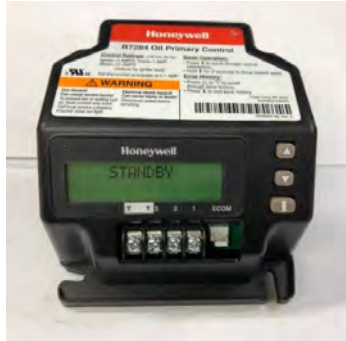
BURNER PRIMARY CONTROL DISPLAY
