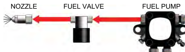
FUEL FLOW DIAGRAM
