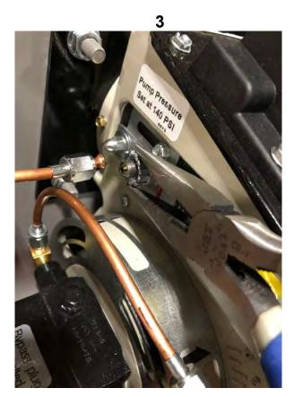
Removed splined nut from burner inlet connection.
