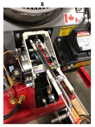
Slide entire drawer assembly out of the burner to reveal the fuel nozzle and electrodes.
