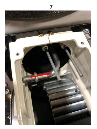
Move drawer assembly to the side in order to slide burner fuel pipe connection out of the housing.
