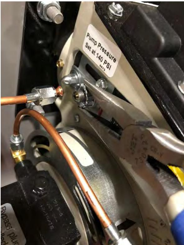
Removed splined nut from burner inlet connection.
