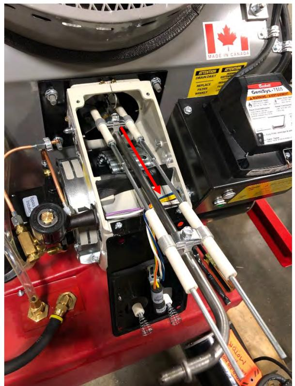
Slide entire drawer assembly out of the burner to reveal the fuel nozzle and electrodes.
