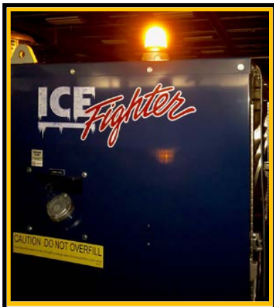
Beacon Displays Steady Amber when Keyswitch is On But Generator is not Supplying 120VAC
