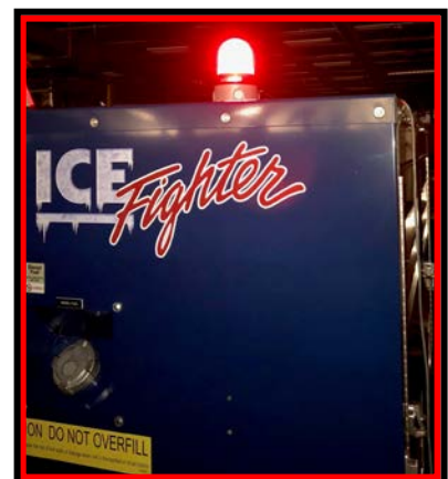
Red Slow Flash Indicates Low Fuel Red Fast Flash Indicates a Heater Lockout Fast Flash rate is selectable at 80/min. or 240/min.
