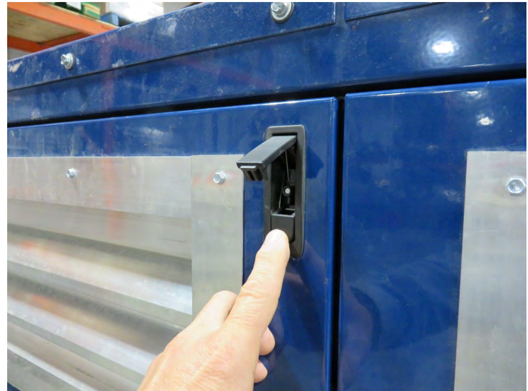
Press Bottom of Latches to Open
