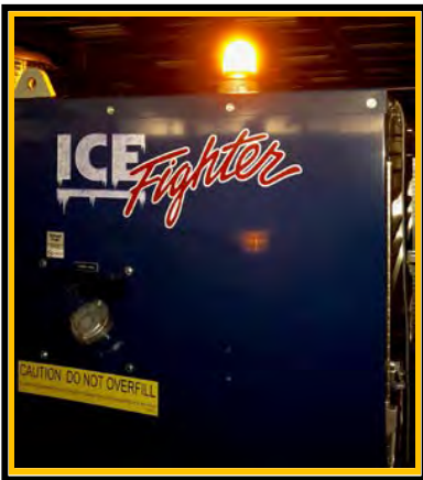
Beacon Displays Steady Amber when Keyswitch is On But Generator is not Supplying 120VAC
