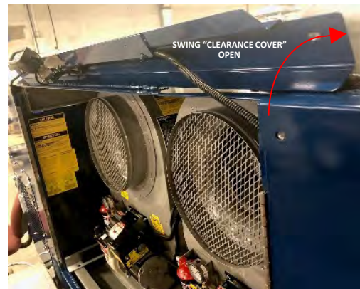
OPENING CLEARANCE COVER TO SLIDE OUT HEATERS
