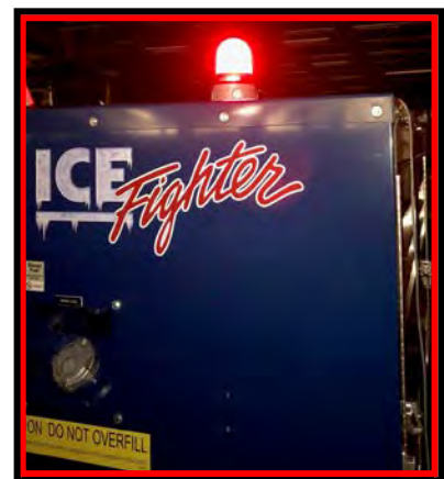
Steady Red Indicates Low Fuel Red Flashing Indicates an alarm state (Heater Lockout) Fast Flash rate is selectable at 80/min. or 240/min.
