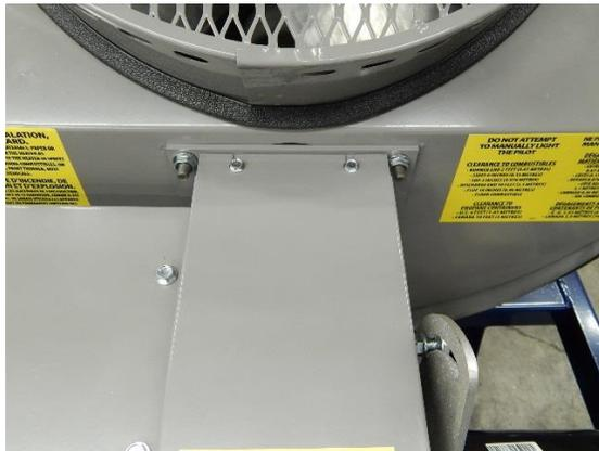
Figure 2: Top two fasteners to loosen
