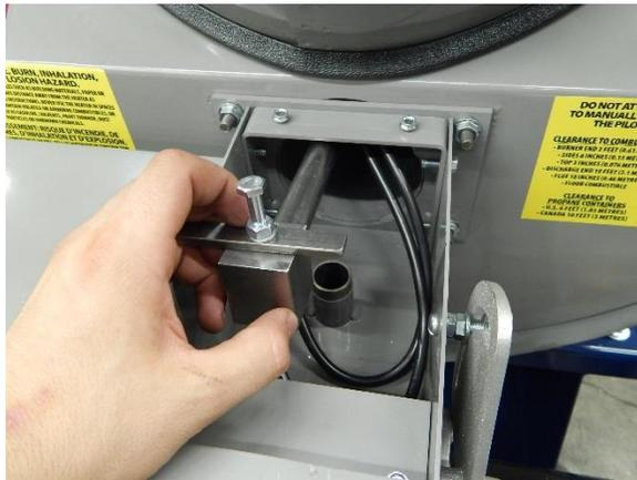
Figure 4: Removal of the electrode drawer assembly
