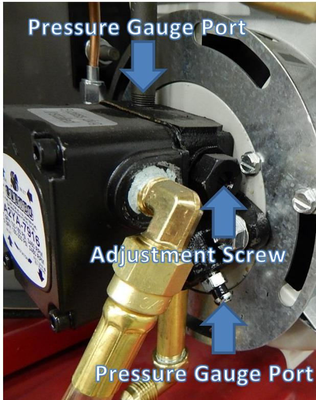
Figure 1: Pressure gauge port and adjustment screw
