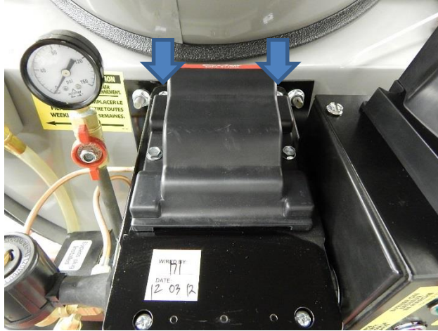
Figure 6: Igniter cover with fasteners indicated
