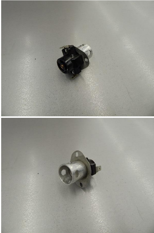
Figure 5: Feeler on opposite end of fan switch
