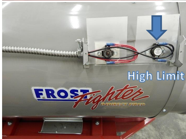
Figure 2: Location of high limit on unit
