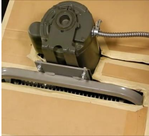
Figure 1: Blocking the fan inlet
