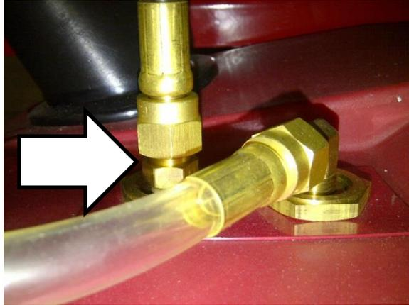
Step 3: Swap the tank bushing from a 90deg to a straight fitting.
