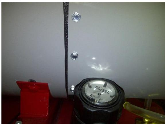
Step 7: Screw the main housing along the side of the jacket.
