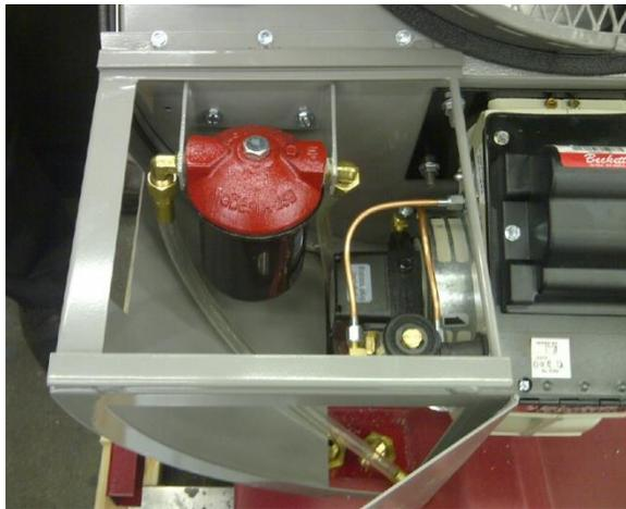
Step 4: Drill 2 holes (13/64" dia.) for filter mount offset approx. 1" towards the burner.
