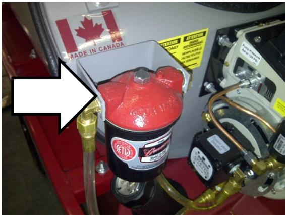
Step 2: Remove the filter & mount
