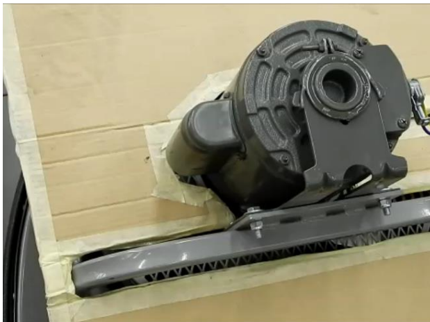
Figure 2: Blocking the fan inlet
